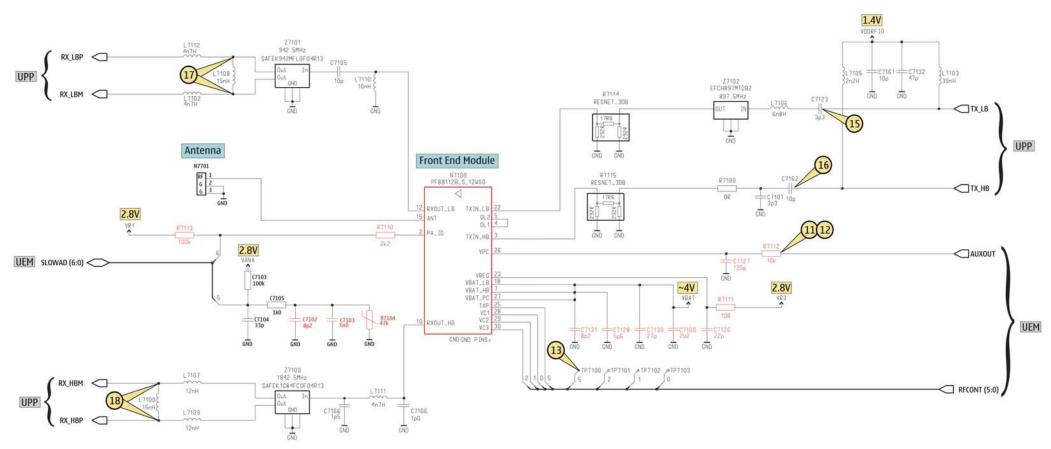
All Components marked in red are NOT reworkable due to shielding!
